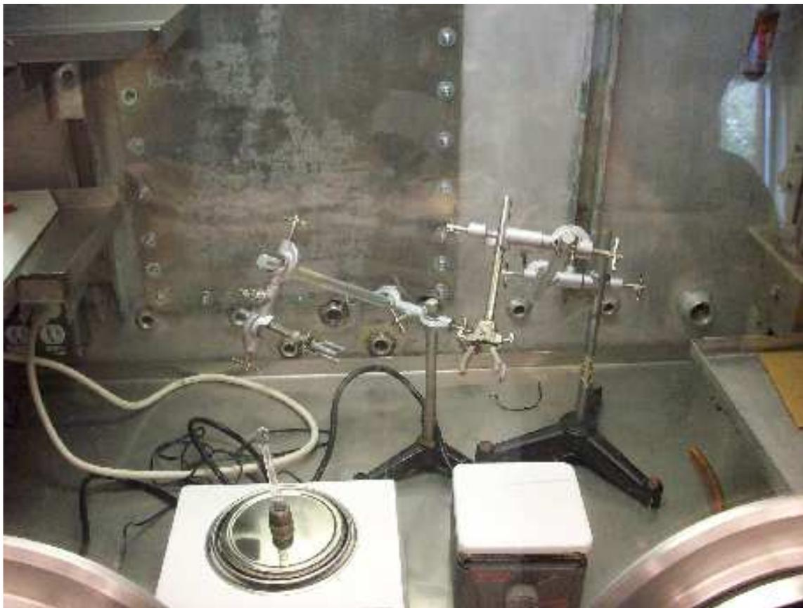
Figure B.3: A photograph of the interior of the glove box. Note the ring stands for holding ampules, as well as the hot plate and scale.
