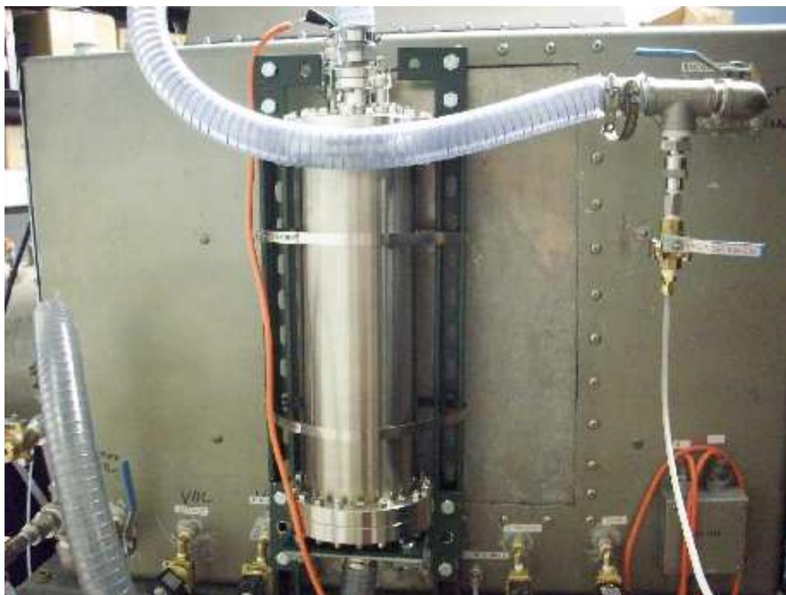
Figure 2.5: Top: a schematic of the plumbing on the rear of the glove box. Bottom: a photograph of the rear of the glove box with the purifying column mounted.
