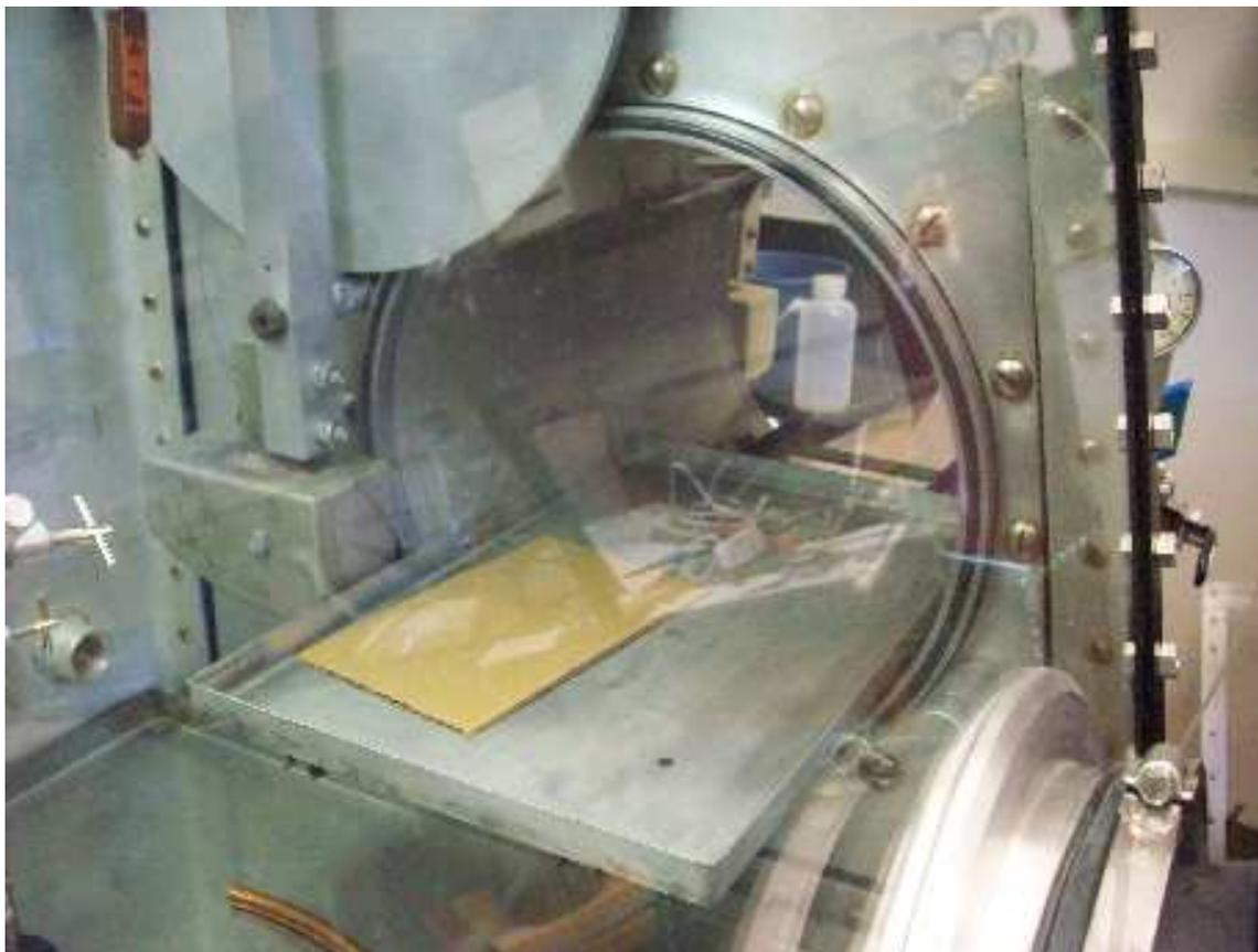
Figure B.5: A photograph of the glove box antechamber with both ends open. Note the sliding tray used to pass materials in and out of the glove box.
