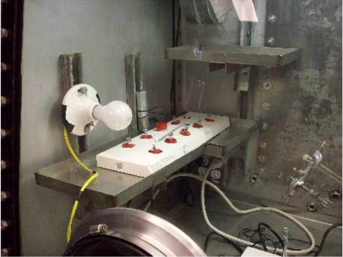
Figure B.4: A photograph of the filaments used to test the purity of the atmosphere. Note the working light bulb in the socket that the filaments will be placed in.
